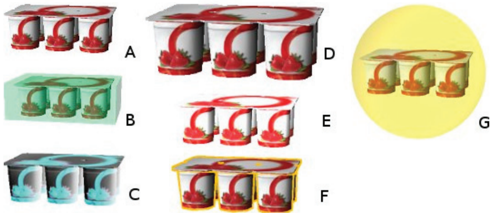
Fig. 3. The six target object strategies to help pointing; A: normal object; B: with rectangular halo; C: with complementary colors; D: enlarged; E: with increased luminance; F: with silhouette edges; G: with spherical halo.
