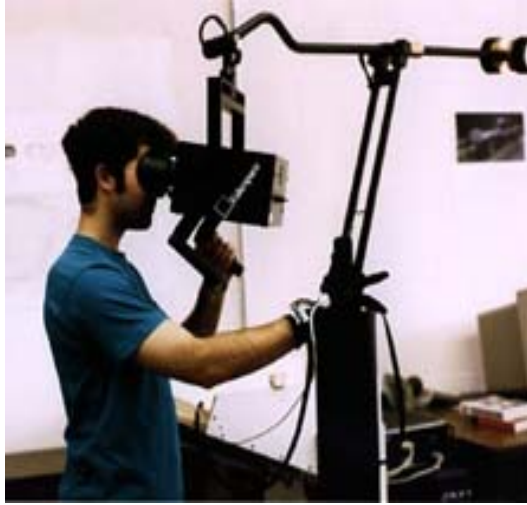
Fig. 2. A binocular omni-orientation monitor (BOOM)
