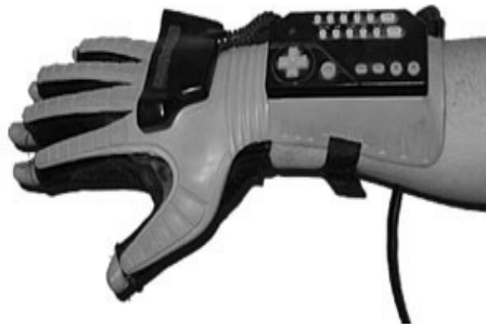
Fig. 5. An instrumented glove (Nintendo power glove)
