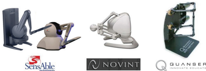
Fig. 2. Commercial haptic devices. On the left, PHANToM haptic devices with 6-DOF by SensAble. On the middle, the FALCON device with 3-DOF by NOVINT. On the right, the Quanser 5-DOF Haptic Wand, by Quanser
